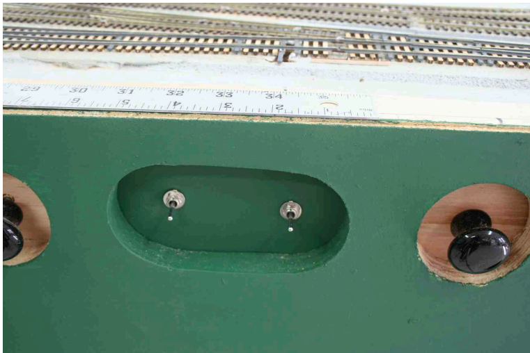
Fascia Switch Controls
